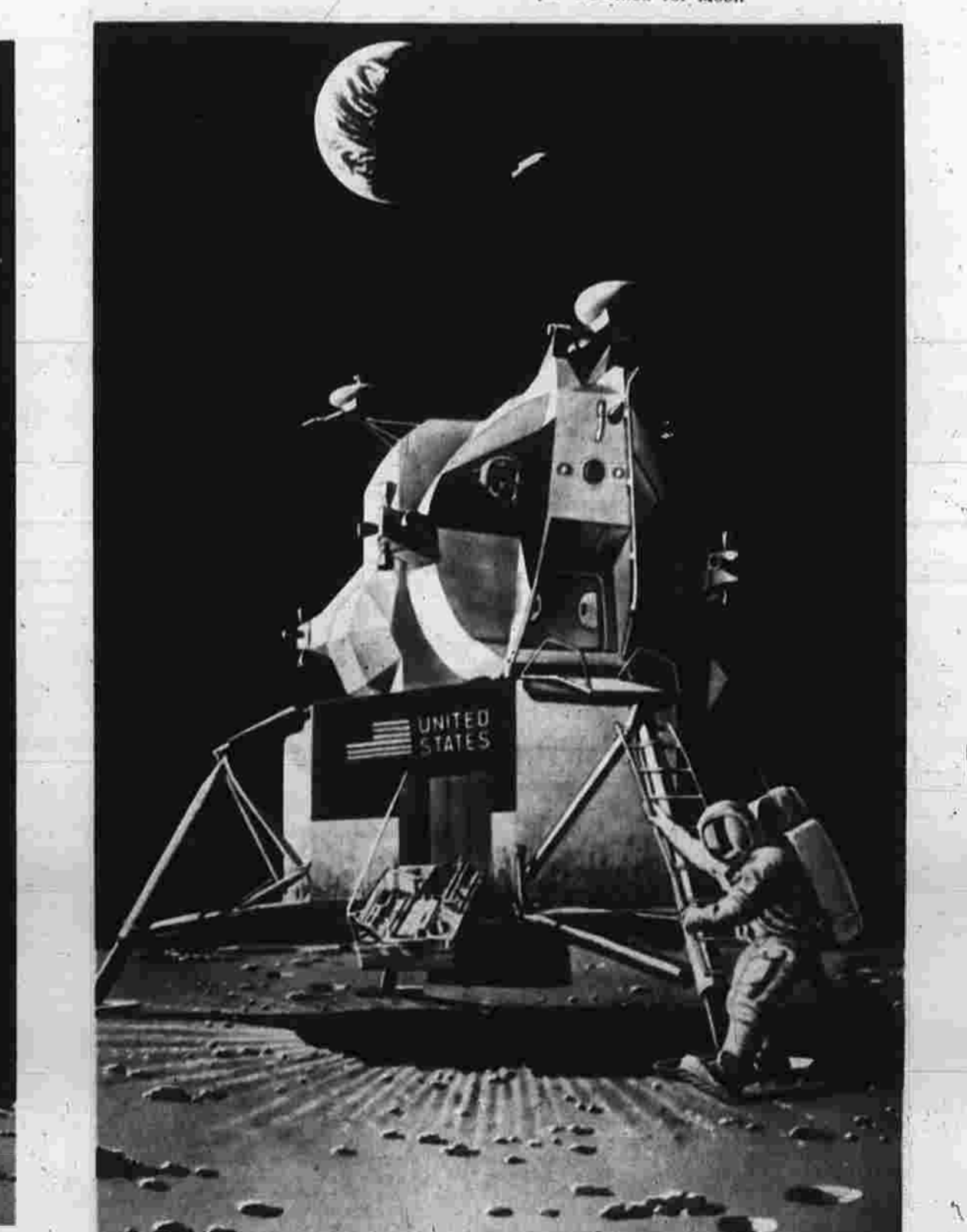
Artist visualizes first step to surface of moon by Apollo 11 Commander Neil A. Armstrong while astronaut Edwin 'Buzz' Aldrin photographs historic event through cabin window. Armstrong will descend ladder on forward landing leg, pulling handle to open equipment bay (center) and triggering TV camera set to transmit live pictures to earth. (Drawing by Los Angeles Times artist Russell Aramsmith.)
